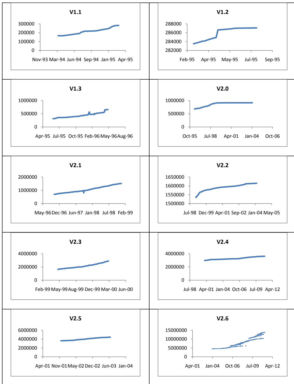
Figure 6.2. LOC growth in Linux, with a total 974 versions.
